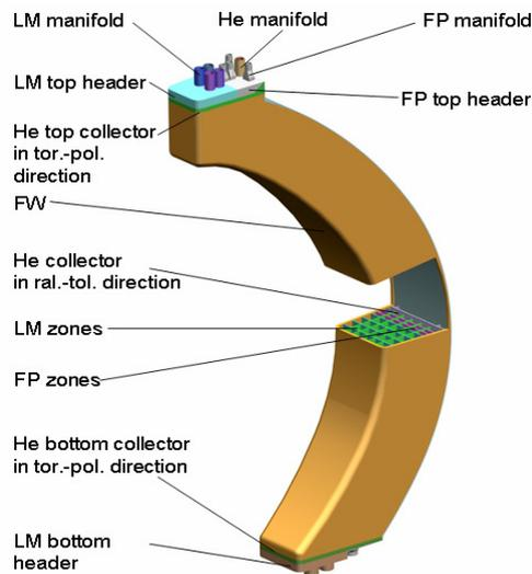
Fig.2 Reference module of DWT-CPL blanket
