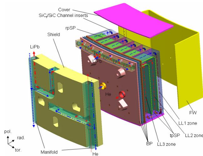
*Fig.4 The exploded view of DLL equatorial outboard blanket module*
