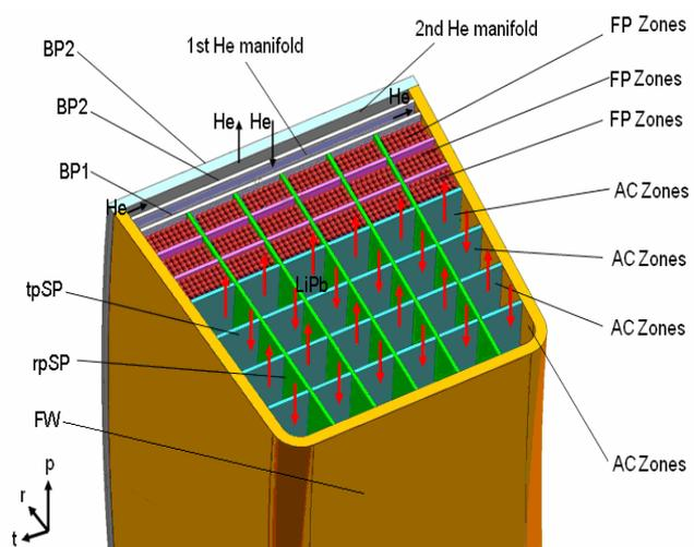
Fig.3 He-gas/liquid LiPb dual-cooled structure of DWT-CPL blanket
