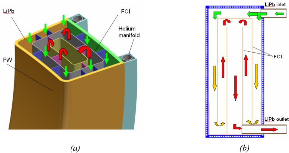
*Fig.5. Schematic layout of blanket structure and LiPb flow channel*
